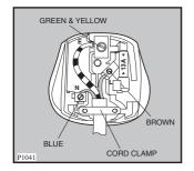
The wire coloured green and yellow must be connected to the terminal marked with the letter «E» or by the earth symbol  $\frac{1}{2}$  or coloured green and yellow.
